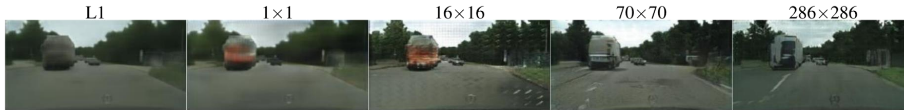
Figure 6: Patch size variations. Uncertainty in the output manifests itself differently for different loss functions. Uncertain regions become blurry and desaturated under L1. The 1 \times 1 PixelGAN encourages greater color diversity but has no effect on spatial statistics. The 16 \times 16 PatchGAN creates locally sharp results, but also leads to tiling artifacts beyond the scale it can observe. The 70 \times 70 PatchGAN forces outputs that are sharp, even if incorrect, in both the spatial and spectral (colorfulness) dimensions. The full 286 \times 286 ImageGAN produces results that are visually similar to the 70 \times 70 PatchGAN, but somewhat lower quality according to our FCN-score metric (Table 3). Please see https://phillipi.github.io/pix2pix/ for additional examples.
